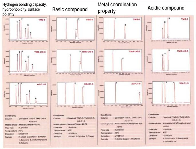
Develosil XG-C1 shows good separation as compared with C1 conventional column.
