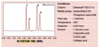
In C18, the organic acid which is hard to separate can also be divided finely.
