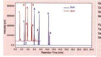
Drugs are analyzed by gradient elution. By using particle diameter 3um, analytical time is shortened sharply.
