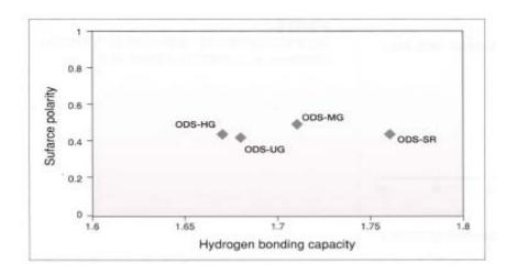
Hydrophobicity is a parameter influenced by the carbon content. ODS-MG which has influence of the base material physical properties to be used, and has 15% of carbon content shows hydrophobicity higher than ODS-UG and HG from the size of the surface area.
